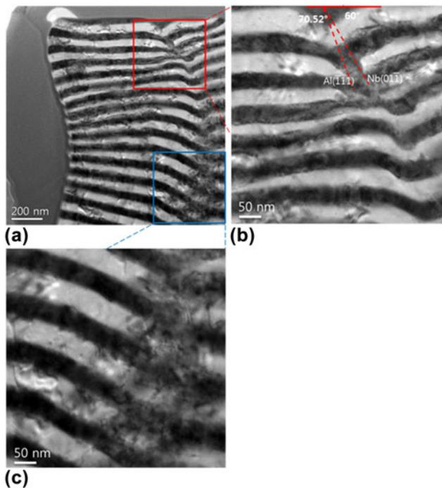
FIG. 7. (a) Cross-sectional BF TEM image of deformed pillar at low magnification, higher magnification view of the regions of macroshear that are highlighted in (b) red box and (c) blue box for the 50 nm Al/50 nm Nb specimen.
