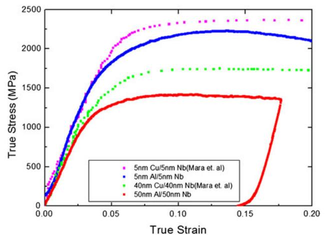
FIG. 5. The stress versus strain plot of Al-Nb pillars with 5 nm Al/5 nm Nb and 50 nm Al/50 nm Nb thickness and Cu-Nb with 5 nm Cu/5 nm Nb and 40 nm Cu/40 nm Nb layer thickness.
