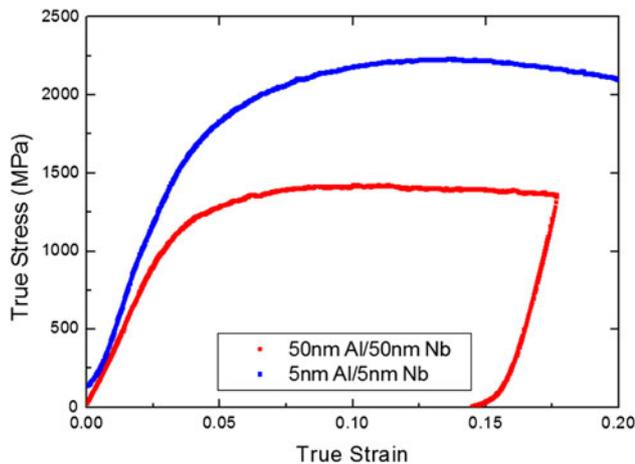
FIG. 3. The stress versus strain plot for the micropillars synthesized from the Al-Nb multilayers with 5 nm Al/5 nm Nb and 50 nm Al/50 nm Nb layer thicknesses.
