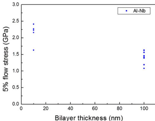
FIG. 4. The 5% flow stress versus bilayer thickness plot showing that the Al-Nb specimen strength is increased with decreased bilayer spacing.
