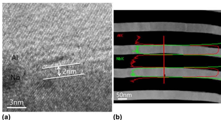
FIG. 6. (a) HRTEM image of Al-Nb interface showing that the thickness of the intermixing is 2.0 nm. (b) Scanning transmission electron microscopy image of Al-Nb layers and the EDS line profile across the interface showing that the average distance of intermixing is 3.5 nm for the 50 nm Al/50 nm Nb specimen.
