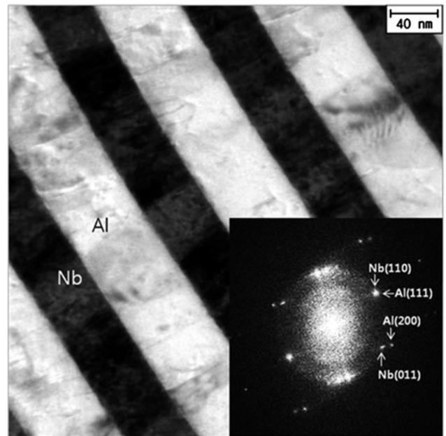
FIG. 1. Bright-field TEM (BF TEM) for the Al-Nb multilayers with 50 nm Al/50 nm Nb layer spacing. The selected area diffraction in the inset confirms the {111} Al//{110} Nb Kurdjumov-Sachs orientation relationship.
