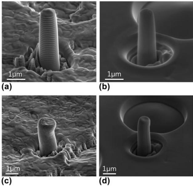
FIG. 2. SEM micrographs of pillars. (a) 50 nm Al/50 nm Nb layer thickness and (b) 5 nm Al/5 nm Nb layer thickness micropillar before compression. (c) 50 nm Al/50 nm Nb layer thickness and (d) 5 nm Al/5 nm Nb layer thickness micropillar after compression.
