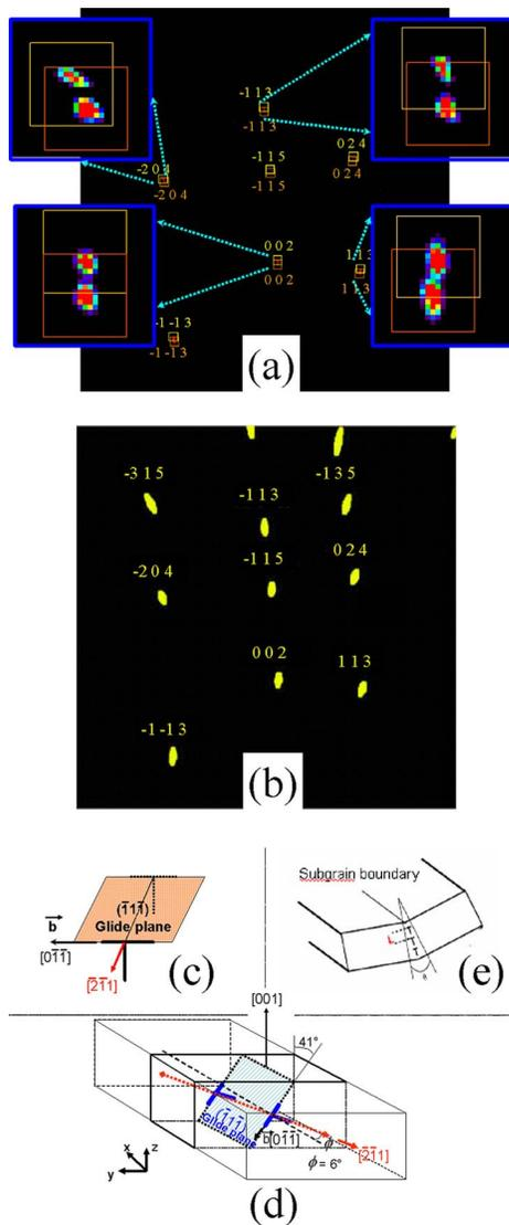
FIG. 3. (Color online) (a) Laue reflection spots at the initial stage (orange) and after they split into the second set of reflection spots (yellow). (b) Simulation of the same initial set of reflection spots based on a particular slip system showing a match with experiment. (c) The active slip system for which the simulation predicts the movement of reflection spots correctly. (d) Modeling of slip deformation in grain 2. (e) Illustration of subgrain boundary formation through polygonization.
