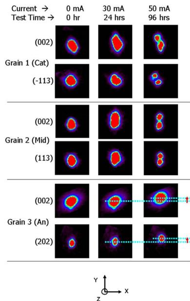
FIG. 1. (Color online) Evolution of Laue diffraction spots (in  $q$  space) of three grains (one at the cathode end, another in the middle, and the last one at the anode end of the line) during an *in situ* EM experiment. For each reflection, the area of  $q$  space is kept constant with length of each side of  $0.03 \text{ \AA}^{-1}$ . Following the evolution of each spot, the reference location is kept constant.
