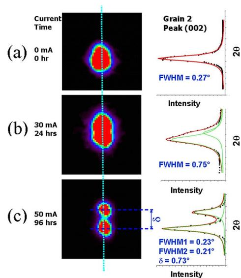
FIG. 2. (Color online) Quantitative measurement of the evolution of a Laue diffraction spot of grain 2 of the three grains mentioned above during an *in situ* EM experiment. Broadening is shown as the spot evolves from (a) to (b), while peak splitting, signifying the formation of low-angle grain boundaries, is evident in (c) as EM progresses.
