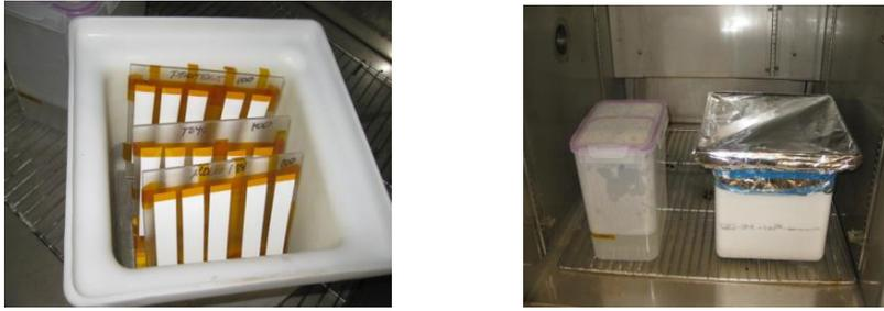
Fig. 1. (a) Backsheet stripes; (b) Backsheet stripes in test chamber
