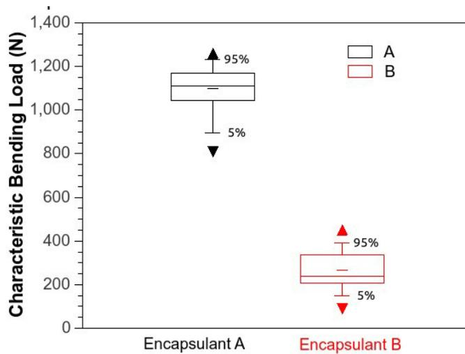
**Fig. 6: Fracture results of solar PV encapsulated with materials A and B**
