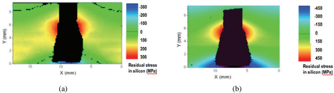
**Fig. 4: Residual stress map of silicon cell near the solder joint of solar PV module, laminated with a. Material A, and b. Material B.**
