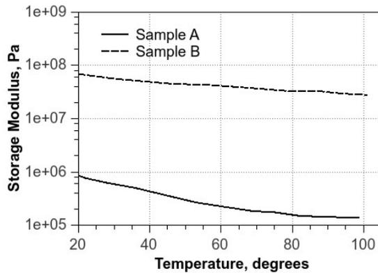
(c) Representative DMA (tension mode) curve of storage modulus vs. temperature
