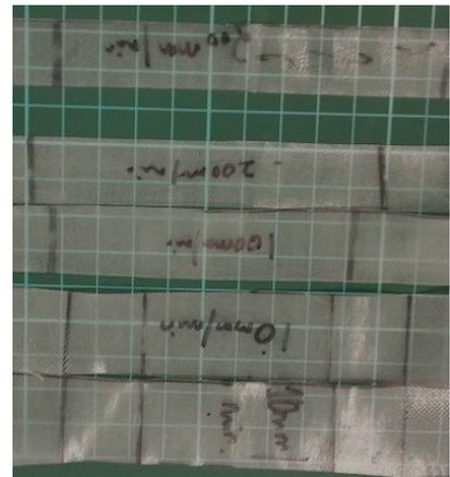
(b) Samples at the end of the test.
