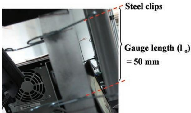
(a) Extensometer (steel clips) mounted at the gauge length.
