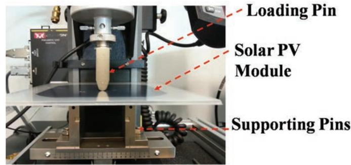
**Fig. 3: Three Point Bending Test Set-up**
