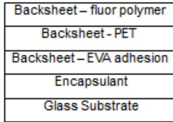
Fig. 4. Test Specimen lay-up consisting of backsheets, encapsulant and glass substrate.
