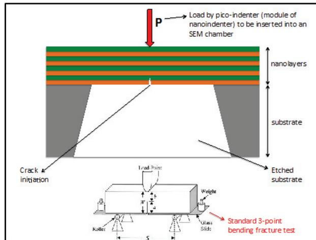
Fig. 1. A proposed novel in situ micro-fracture testing for nanostructured materials/films enabled only by recent advances in nanomaterials characterization and manipulation tools such as FIB (Focused Ion Beam) and a Pico-Indenter (recent advances in Nano indentation tooling) as well as MEMS techniques such as etching of substrates and building of cantilever structures
