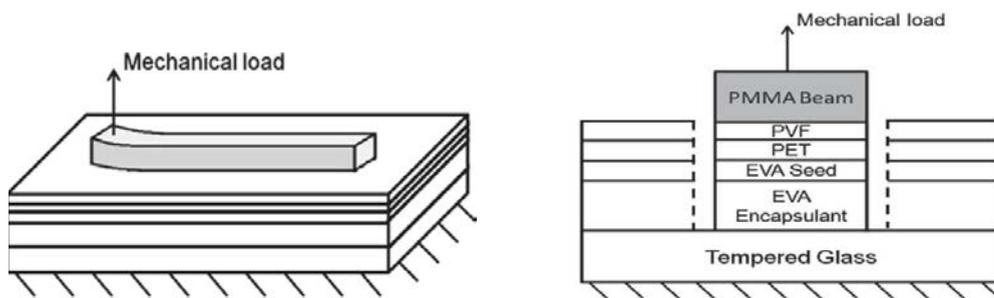
(a) PMMA beam attached to the backsheet surface;
