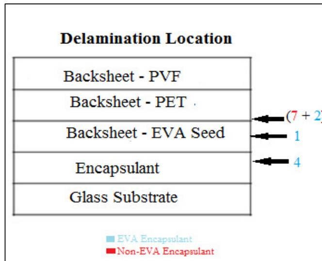
Fig. 9. Delamination location for both the samples. (Red colour indicating the sample 1 with EVA encapsulant and blue colour for sample 2 with non-EVA encapsulant)
