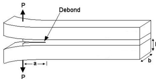
Fig. 3. Double Cantilever Beam test method.
