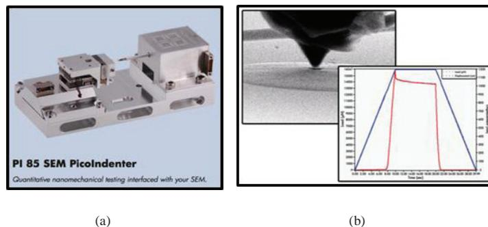
Fig. 2. . Nanomechanical tester that can be interfaced within an SEM environment (a) would allow mechanical data to be fully synchronized (b) with the SEM video (in situ observation) revealing unique insights that could lead to complete understanding of materials behaviours at the nanoscales (Courtesy of Hysitron Inc.)
