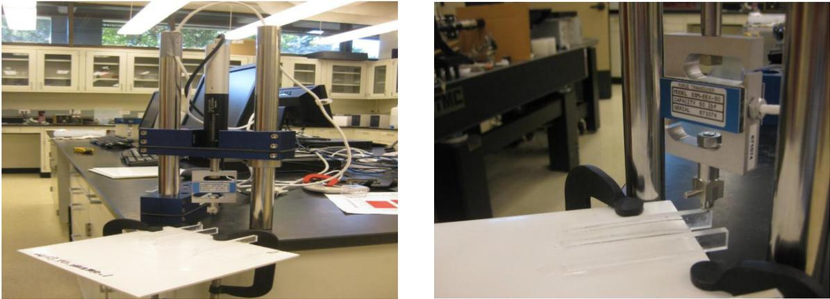
Fig. 6. The test set up showing the laminate sample fixed to the testing table with C-clamp, the PMMA beam attached to the backsheet surface and the loading tab. The loading tab is connected to the Delaminator v8.2 adhesion testing system.
