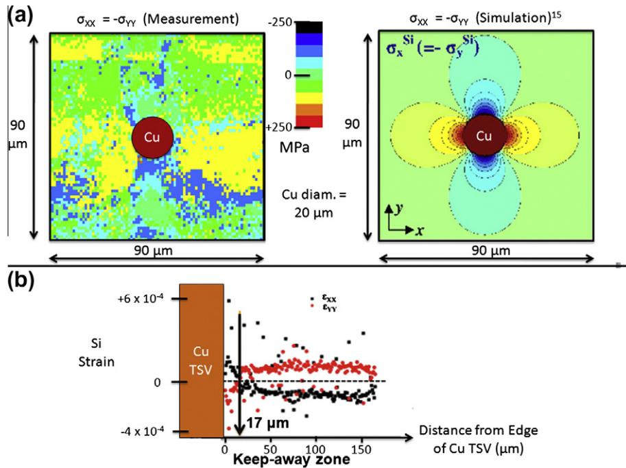
**Fig. 4.** Si stress state surrounding the Cu TSV showing (a) the measured stress map from the top of the TSV sample as compared to the simulation result performed by other research group [17] and (b) the strain/stress profile from the side of the TSV sample showing the “keep-away” zone from the edge of the Cu TSV of about 17  $\mu\text{m}$ .
