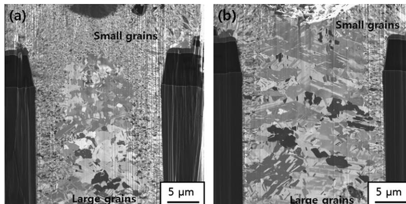
**Fig. 3.** FIB images showing (a) cross-section of a Cu TSV in the as-received state (approximately two months after the Cu deposition into the TSV structures) and (b) cross-section of another Cu TSV in the post-annealed state (after annealing of 200 °C for 1 h). These images indicate significant grain growth during the annealing phase of 200 °C for 1 h.
