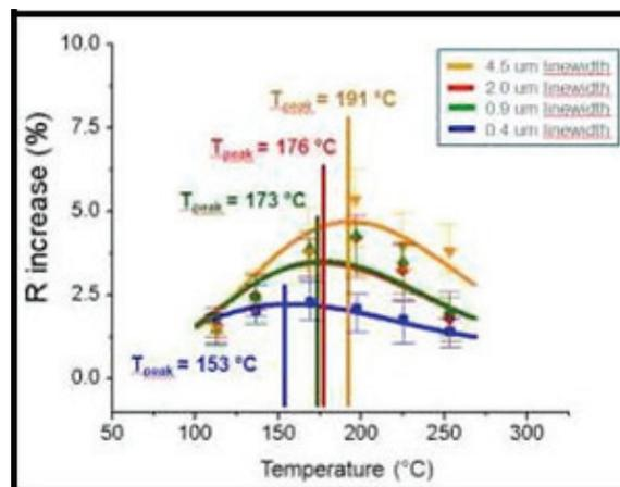
Fig. 2. Stress Migration temperature profiles for Cu samples with different linewidths. The data point represents the median value while the error bar represents the range of all data (10 DUT's per test temperature per linewidth).
