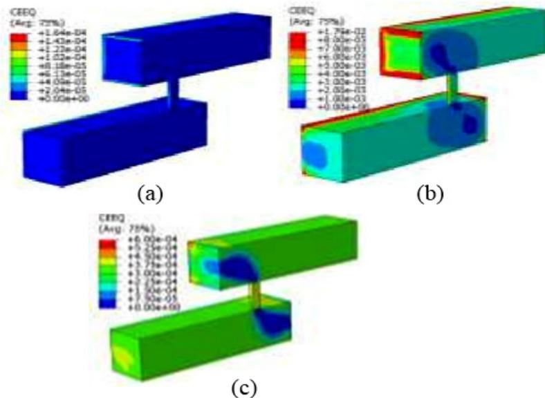
Fig. 5. Simulated equivalent creep strain in the Cu lines and via after 100 h at (a) 20 °C, (b) 200 °C and (c) 350 °C.
