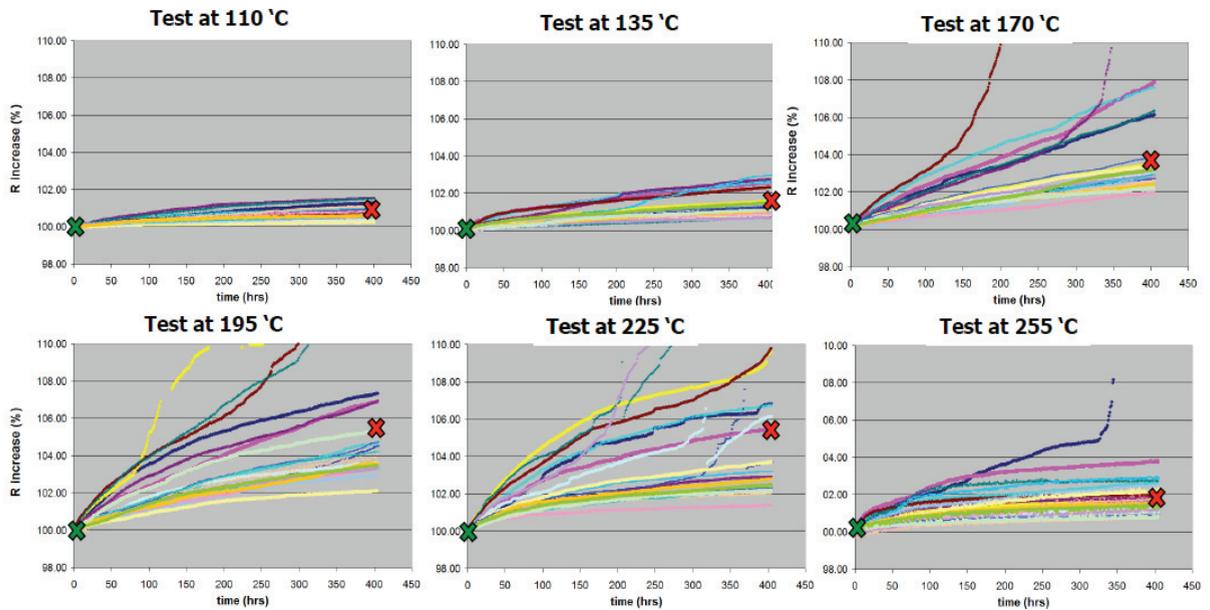
Fig. 1. Typical SM Test Measurements:  $\Delta R/R$  vs. Time
