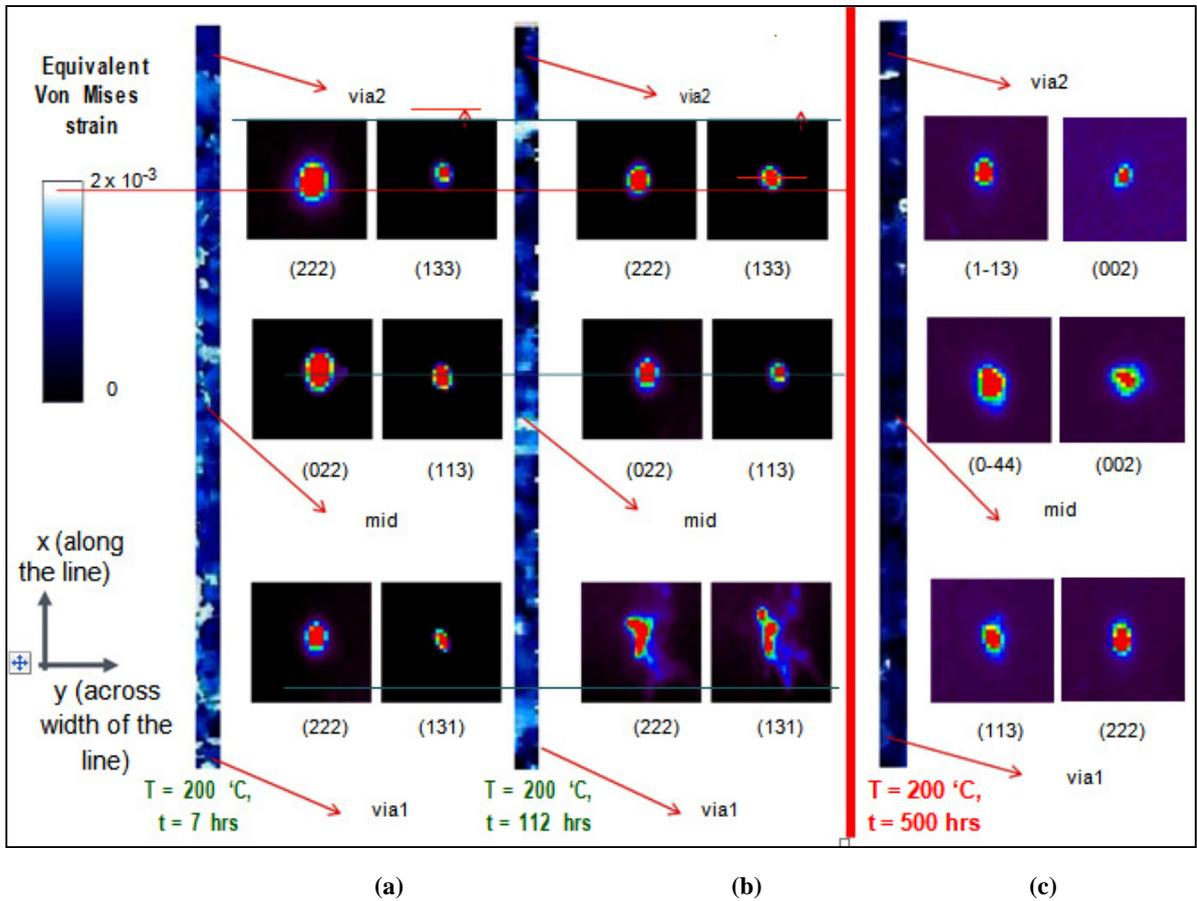
Fig. 4. . Complete evolution of a Cu interconnect line (2um width, 20um length), which is the same interconnect line in Figure 3, in terms of von Mises strains and Cu Laue reflection peak shapes during a 500-hrs thermal loading/baking experiment; (a) at time equals to 7 hrs, (b) at time equals to 112 hrs and finally (c) at time equals to 500 hrs of the thermal loading/baking experiment.
