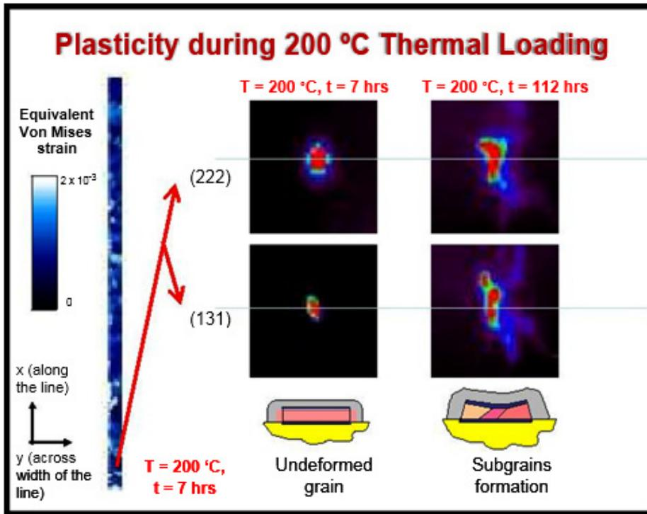
Fig. 3. Plasticity during 200°C thermal loading in 2  $\mu\text{m}$ -wide interconnect line. Streaked (asymmetrically broadened) Cu Laue peaks were observed in one end of the M2 line segment (length = 20  $\mu\text{m}$ ) just above the via as shown above (red arrow) after about 100 hrs of thermal loading. Similar observation was found with the 4.5  $\mu\text{m}$ -wide sample.
