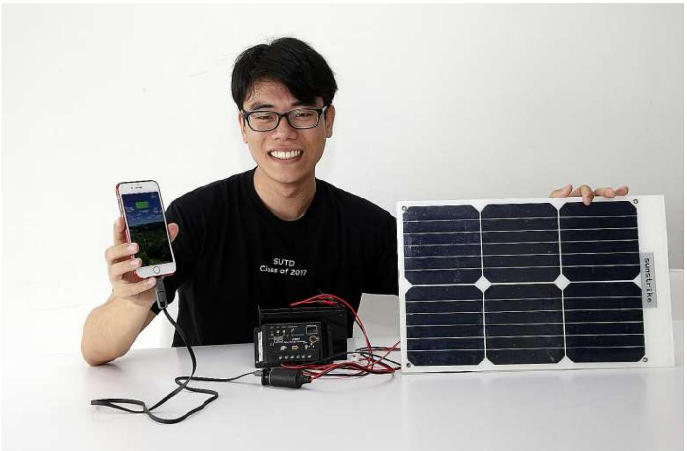
Mr Tan's charger consists of an A4-sized solar panel, a battery to store the power and a controller to regulate the charging. It can generate enough energy in a day to power an iPhone for at least two full charges. ST PHOTO: CHEW SENG KIM
