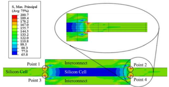
Fig. 6. Maximum principal stresses (MPa) in silicon cell postsoldering.
