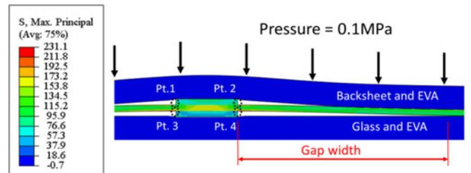
Fig. 9. Stress distribution and cell deformation at the end of the evacuation step. Note the gaps on both sides of the interconnects.
