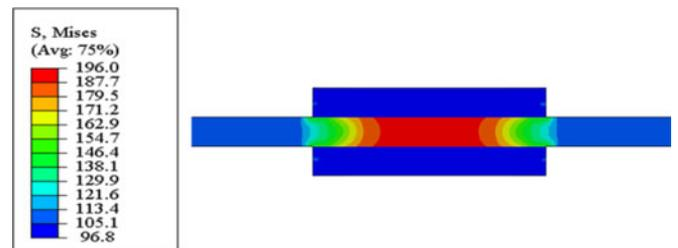
Fig. 8. Von mises stress (MPa) distribution in copper interconnects at 25 °C postsoldering.
