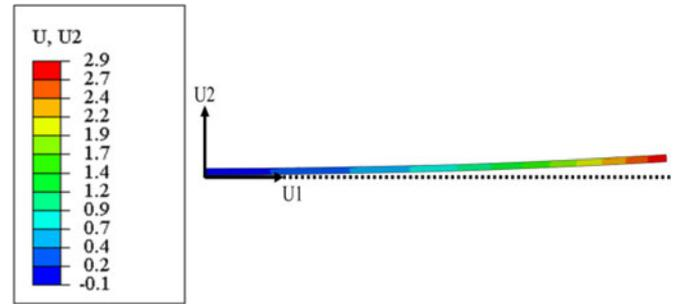
Fig. 11. Warpage of PV laminate at the end of the manufacturing cycle (dimensions in mm).
