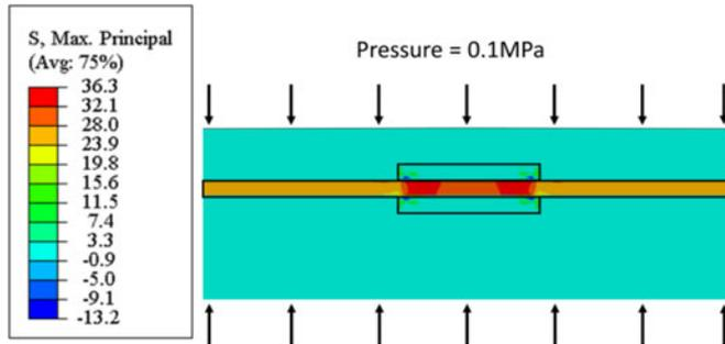
Fig. 10. Cured EVA encapsulating the silicon cell and interconnects with the application of 0.1 MPa at 150 °C (stresses in MPa).
