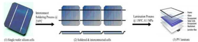
Fig. 2. Typical manufacturing cycle of a conventional wafer-based PV laminate. [5].
