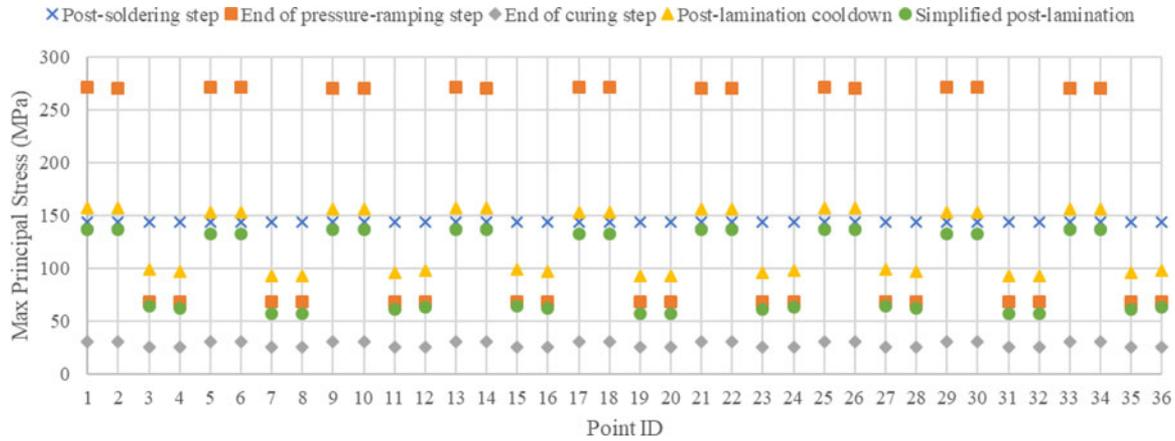
Fig. 7. Plot of maximum principal stress at 36 critical points in three cells throughout the manufacturing process.
