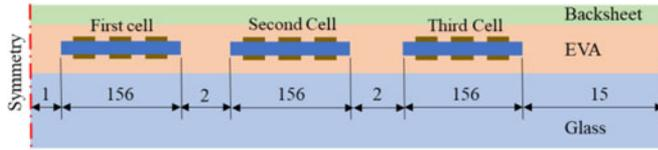
Fig. 5. Cross-sectional view of the PV laminate along A–A. (Not to scale).
