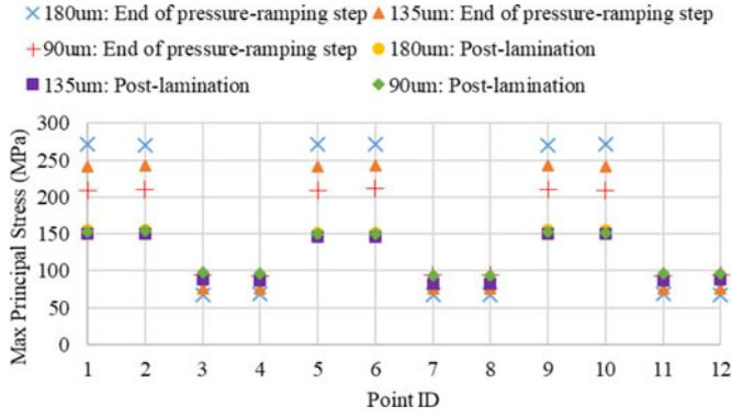
Fig. 12. Plot of maximum principal stresses for cells of different thickness at the end of the evacuation and postlamination cooldown steps.
