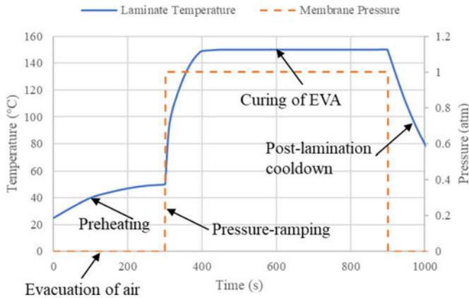
Fig. 3. Variation of pressure differential and temperature in a laminator during the lamination process.
