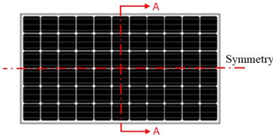
Fig. 4. Plan view of a typical conventional 66-cell silicon-wafer-based PV laminate [picture taken from public domain].
