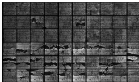
Fig. 1. Typical EL image of a PV module showing that the majority of cracks (dark regions) in silicon cells occur along the edges of the interconnects [2].
