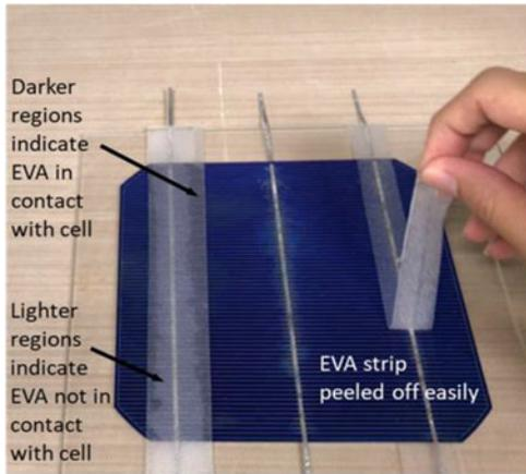
Fig. 13. Experiment verifying assumption of solid EVA during the evacuation step in the lamination process.
